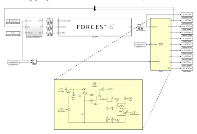
In the grey box in the model depicted above, the three parameters which are the input to the FORCES PRO controller, are calculated.
