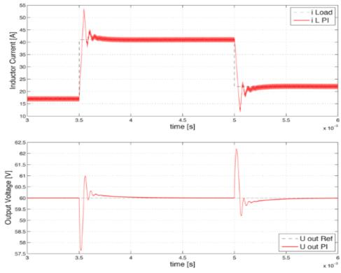
From the figures above one can see that the current in the inductor has a high overshoot and the output voltage has a relatively long settling time when a change in the load resistance occures.
