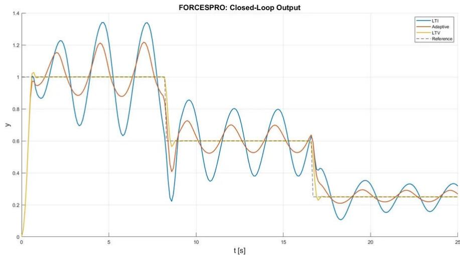
The plant dynamics are varying and unstable, which makes it very challenging for an LTI controller to track the changing setpoints. Both the
